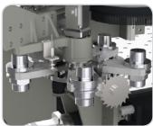
• Rotating Magazine 5 tool capacity, optimum tool change time as it is nearby the spindle.
