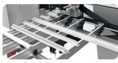
• Output robot conveys the cut profiles on conveyor automatically.
