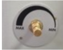
Figure 1 : Hydro-Pneumatic Cylinder Saw Blade Rising Speed Adjustment
